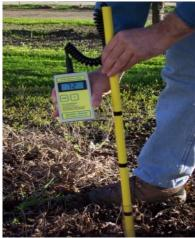
A fast and easy way to take soil moisture measurements in percent soil moisture, using only one moisture sensor for multiple moisture readings over the entire root zone, in any size area. Here is how you do it:
